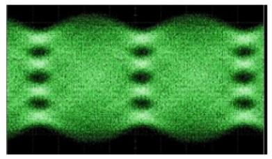
S21 Measurement of MZM and SiGe BiCMOS Driver combination
