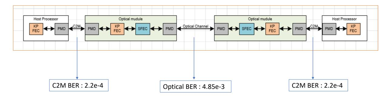
For some of the stringent high loss AUI Channels on the host, we may need to turn on the segmentation FEC proposal to close the link budget.
