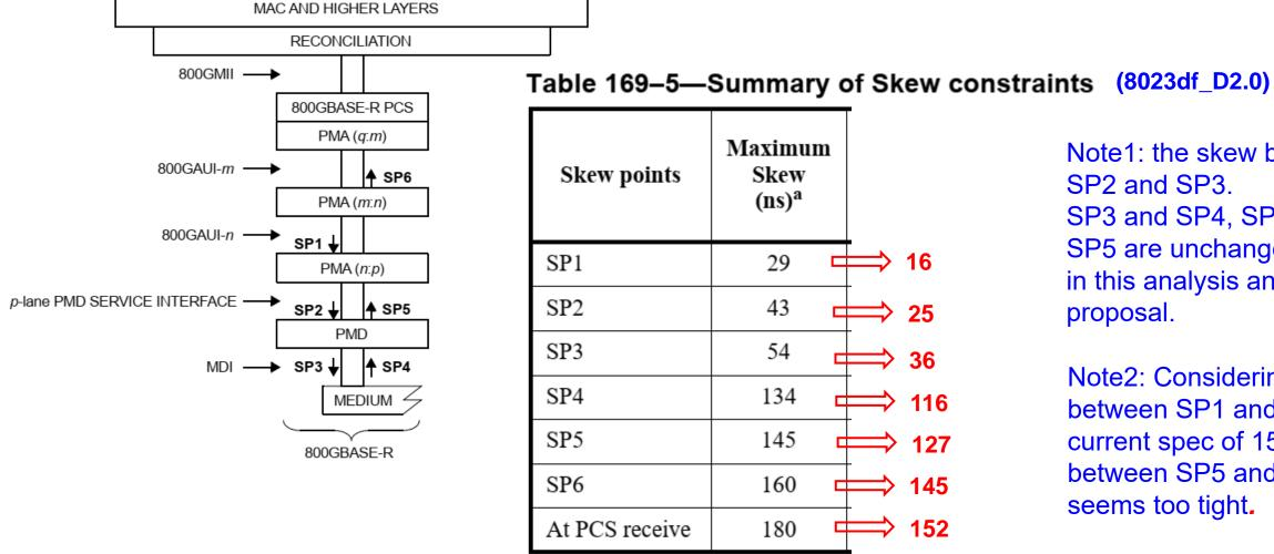
Note1: the skew between SP2 and SP3. SP3 and SP4, SP4 and SP5 are unchanged in this analysis and proposal.
