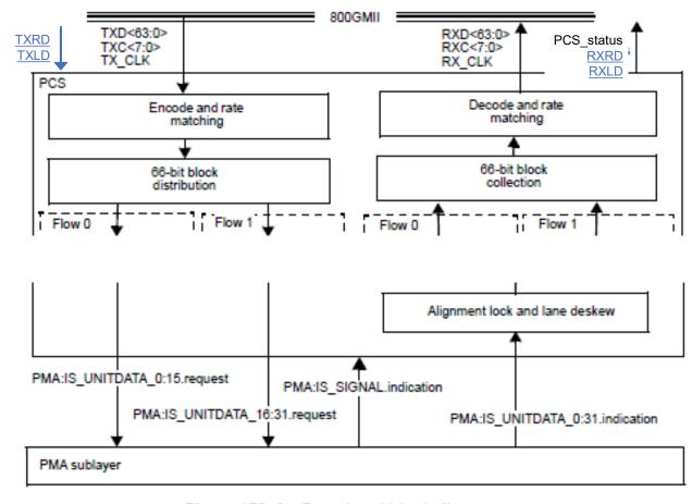
Figure 172-2—Functional block diagram
