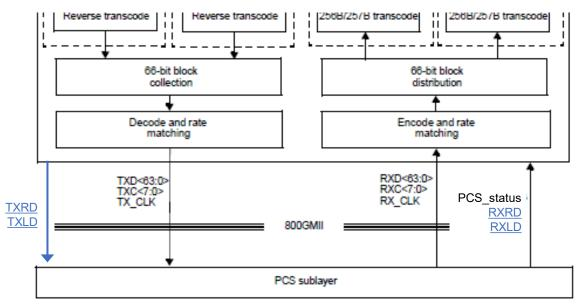
Figure 171-2—Functional block diagram for the PHY 800GXS
