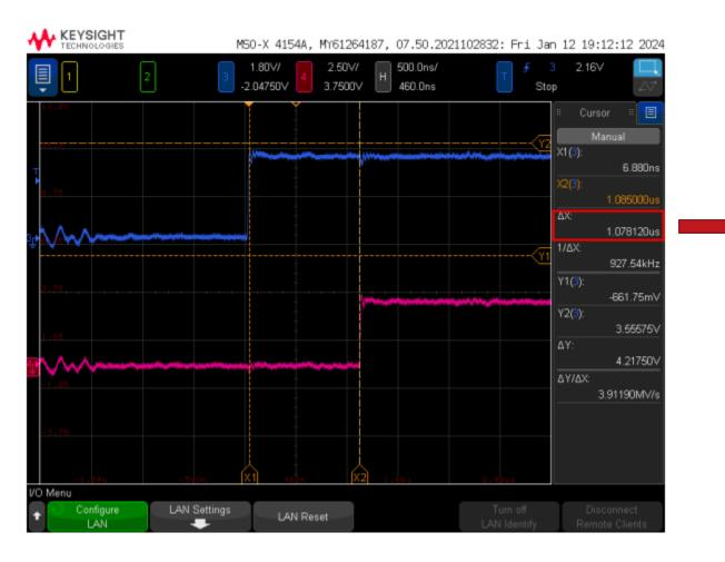
The total latency over 100m cable is measured as 1.08us, which means the pure PHY Tx+Rx latency is around 0.5us. The BER in this case is in the order of 1e-14.
