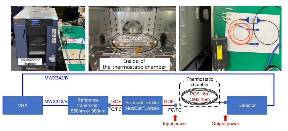
I evaluated the reproducibility of the frequency response measurement with OM3(15m) for reference. Furthermore, I measured the input and output light intensity of OM3 and POF.
