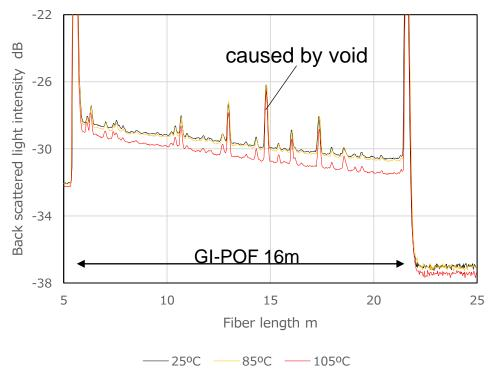
Since the most likely causes of noise are backscattered light and forward scattered light, I re-checked optical time-domain reflection.
