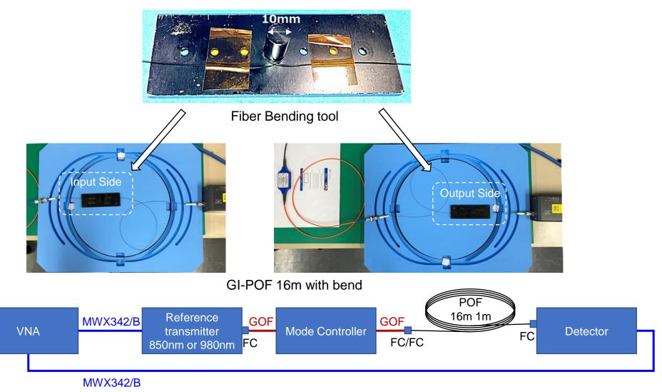
Bending Seems to affect little to the frequency characteristics of the measurement results, considering the reproducibility of the measurement.
