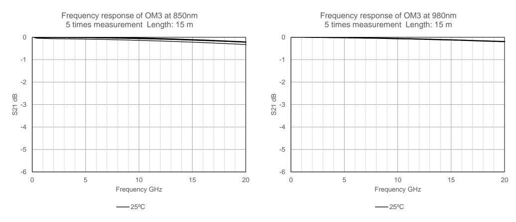
The insertion loss (incl connection and the attenuation) of POF(16m) are higher than those of OM3(15m). But light intensity is sufficient.
