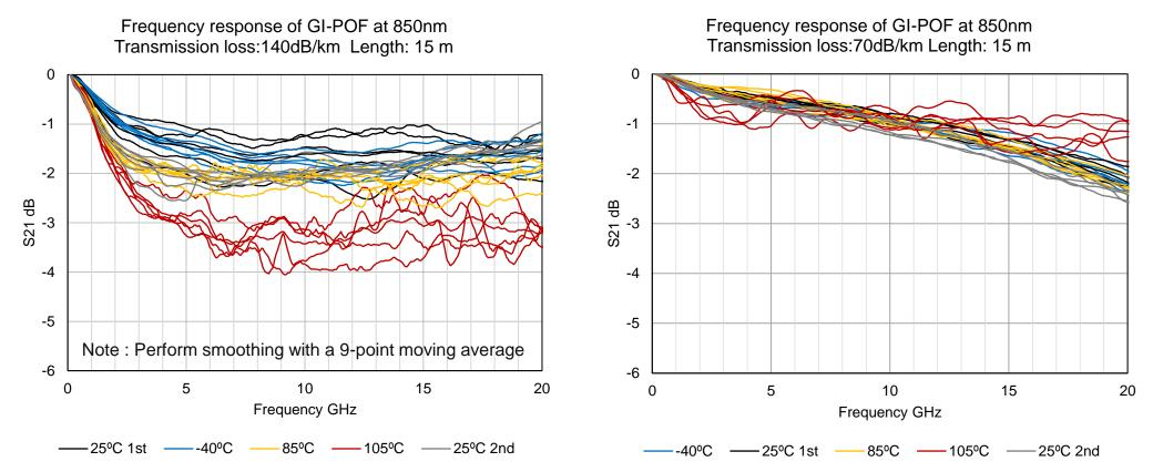
The following graph shows the plots of 30 measurements of frequency response at 105°C. The variation in frequency response has been almost halved.
