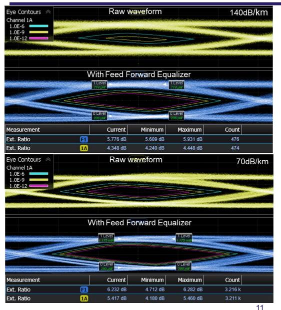
The colored box in the eye diagram indicates the approximate value of the bit error rate calculated from the eye diagram.
