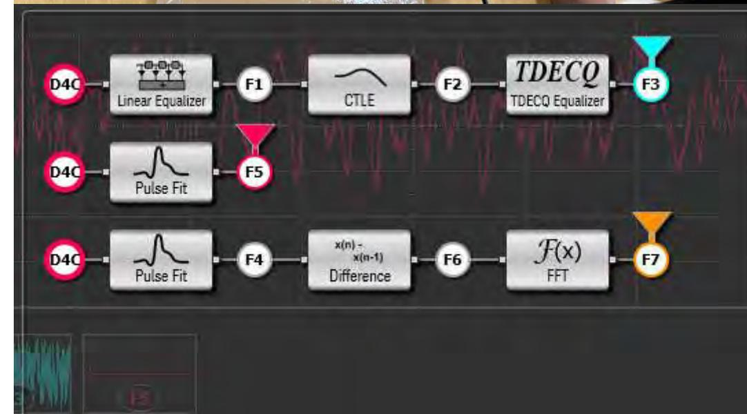
P8023dj: D3: V1.4 Jitter operations (179.9.4.7) at TP1a (33dB) 2024
