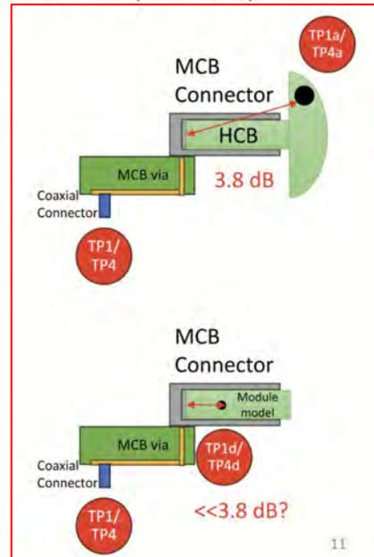
With an allocation of 3.8 dB to the HCB, The insertion loss between TP1d and TP1a is likely about 3 dB (it may be lower if the DSP in the module is packaged).
