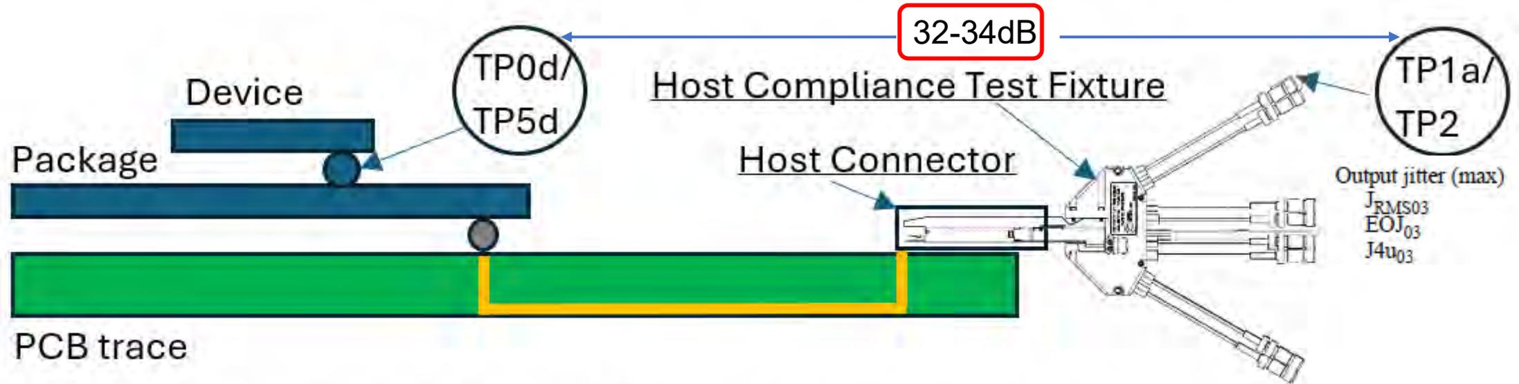
Figure 1: Typical 802.3dj host test point model
