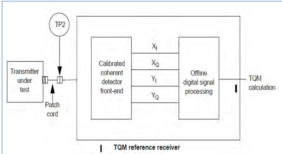
Offline digital signal processing used for TQM calculation
