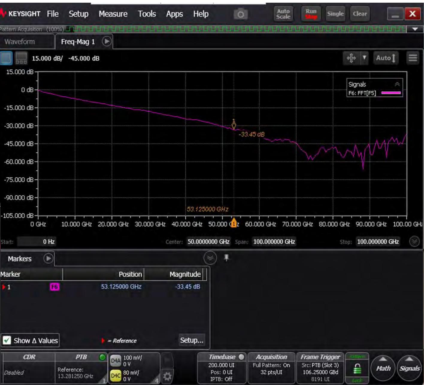
P8023dj: D3: V1.4 Jitter operations (179.9.4.7) at TP1a (33dB) 2024
