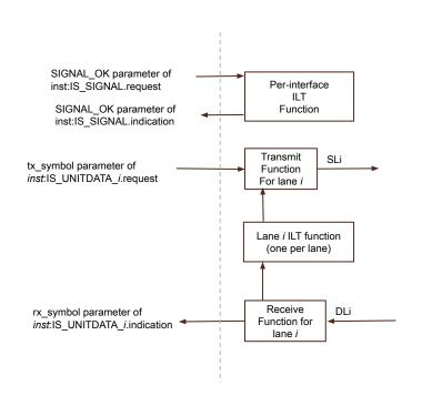
There is a piece missing from the optical block diagram (e.g., Figure 180-2), as well as the electrical block diagrams (e.g., Figure 163-2) relating to the bidirectional nature of ILT. This is relevant to electrical PMDs, optical PMDs, and AUI components.
