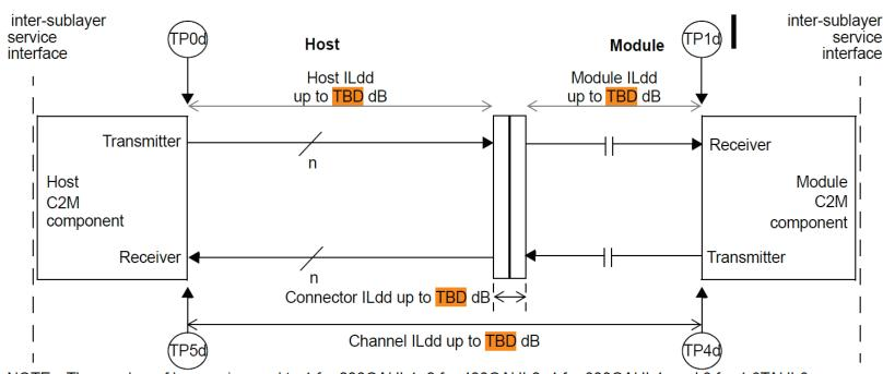
NOTE—The number of lanes n is equal to 1 for 200GAUI-1, 2 for 400GAUI-2, 4 for 800GAUI-4, and 8 for 1.6TAUI-8.
