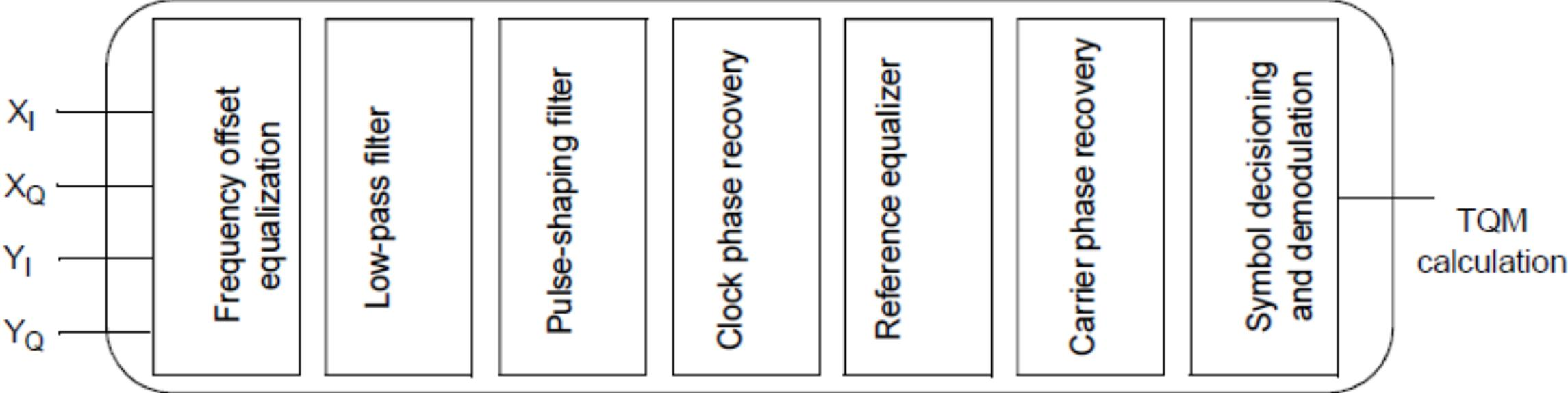
The basic blocks that are required for a reference receiver implementation are illustrated
