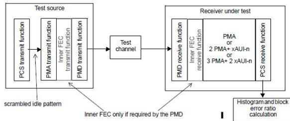
Figure 174A-4—Test configuration for a PHY using PCS counters
