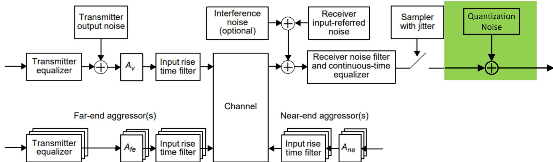
Figure 178A-7—Sources of noise considered in calculation of COM
