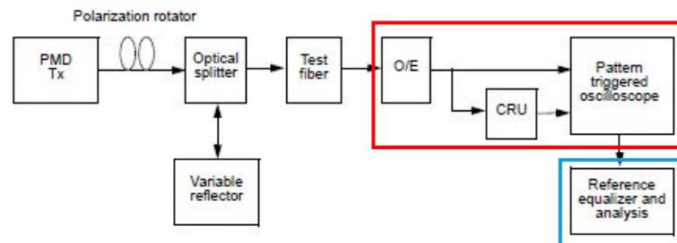
Figure 121-4—TDECQ conformance test block diagram
