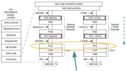
When tx\_mode = DATA the PCS transmit path may use the clock recovered from the PMA above the XS - or -
