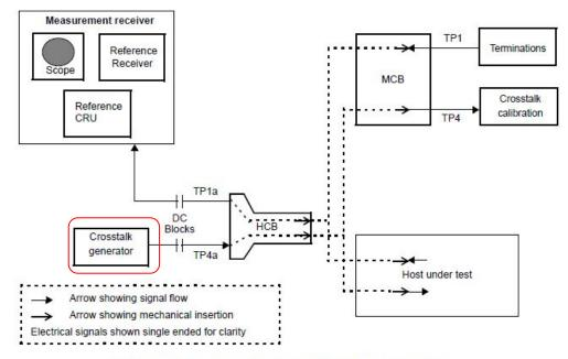
The crosstalk generator output is specified to be an asynchronous pattern with maximum differential peak-to-peak and minimum transition time at TP4. Equalization is not specified.
