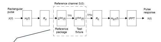
Figure 163A–2—Configuration for transmitter reference steady-state voltage, pulse peak, and ERL
