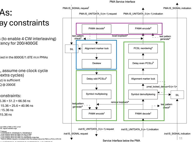
m = 8 (200GBASE-R), 16 (400GBASE-R), 32 (800GBASE-R), or 16 (1.6TBASE-R) n = 1 (200GBASE-R), 2 (400GBASE-R), 4 (800GBASE-R), or 8 (1.6TBASE-R)
