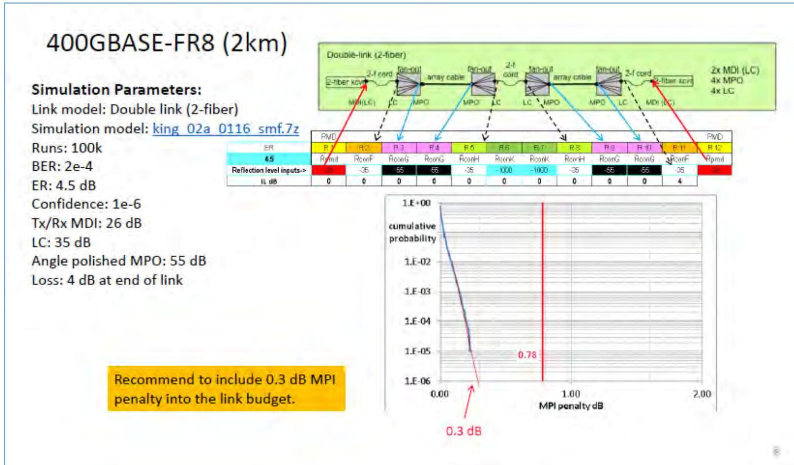
Using the nominal fiber cabling models and reflectance values, Hai-Feng proposed the following MPI penalty allocations for the 802.3bs power budgets:
