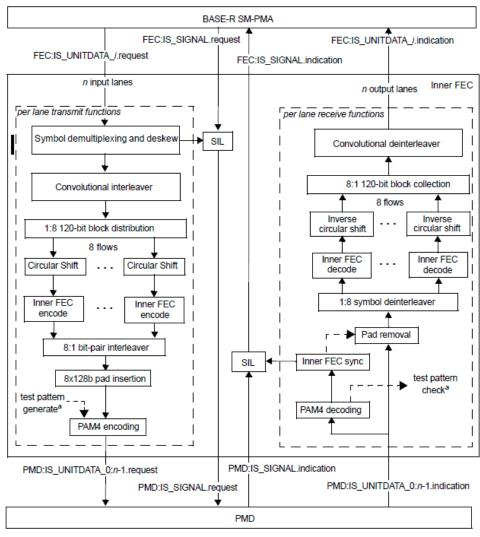
Figure 177-2 shows the test pattern injection point. Injecting the test patterns at this point and further Gray coding them isn't what is intended. However the use of the optional pre-coder within the PAM4 encode process should be documented.
