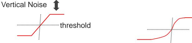
A curved edge amplifies noise-to-jitter conversion, creating more jitter than a linear edge does. (Not trying to model the edge, just adding another param to the model.)
