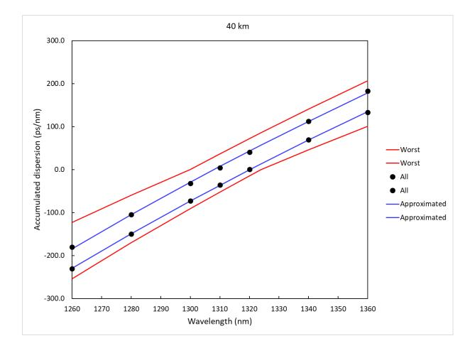
1299 nm min CD = -78.3 ps/nm 1314.5 nm max CD = 22.45 ps/nm
