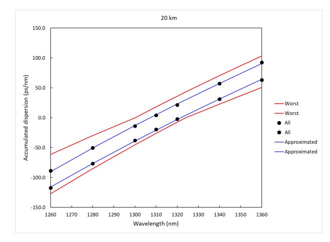
1299 nm min CD = -42.23 ps/nm 1314.5 nm max CD = 14.75 ps/nm
