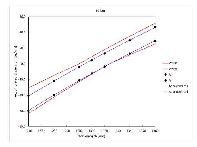
1299 nm min CD = -22.2 ps/nm 1314.5 nm max CD = 8.3 ps/nm
