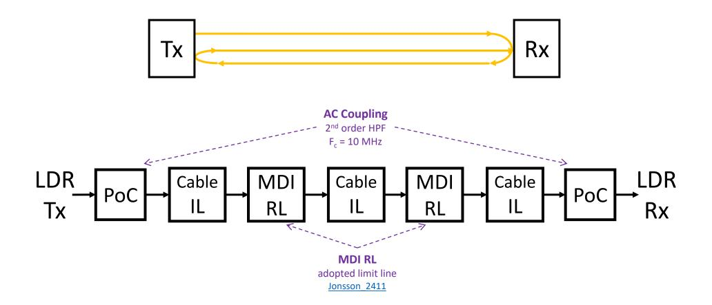
Double reflections are attenuated by 3x of cable loss
