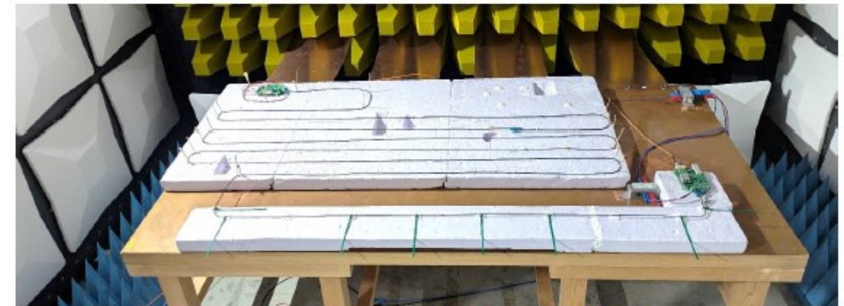
Test set-up, complete arrangement for test channel 1 (12 m)
