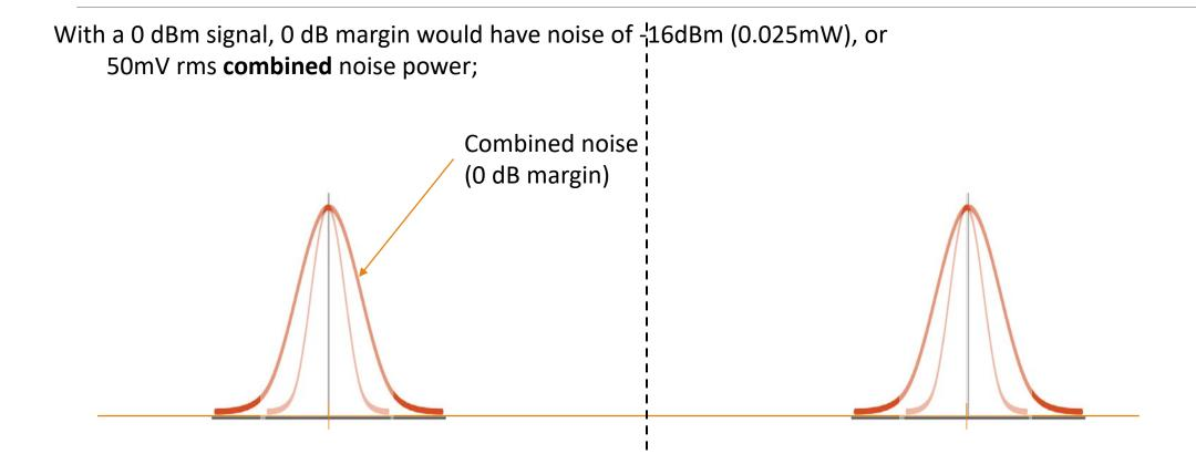
Noise adds *linearly* as power, so 6 dB margin tolerates 49.992mW additional noise 12 dB margin tolerates 49.998mW only 7 *micro*Watts more.
