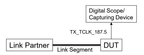
For Jitter measurements, the measurement BW of the capturing device shall be more than 200MHz.
