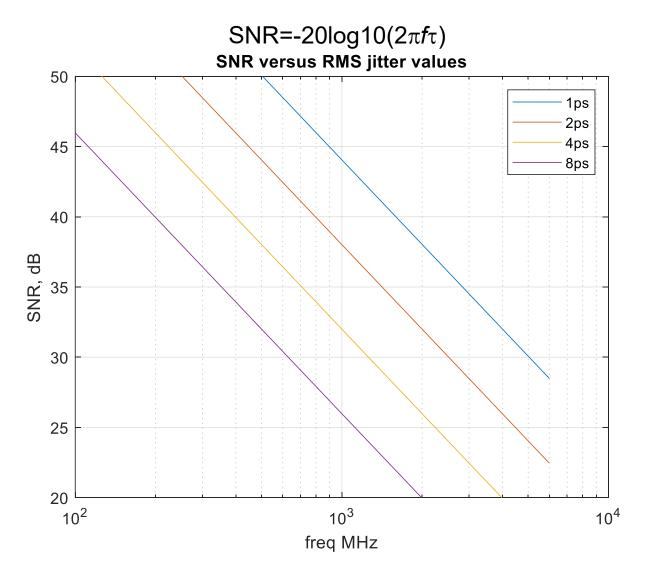
For a wideband signal, geometric mean of SNR from 10 % of Nyquist to Nyquist calculated to be:
