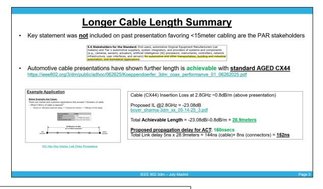
Cable (CX44) Insertion Loss at 2.8GHz ~0.8dB/m
