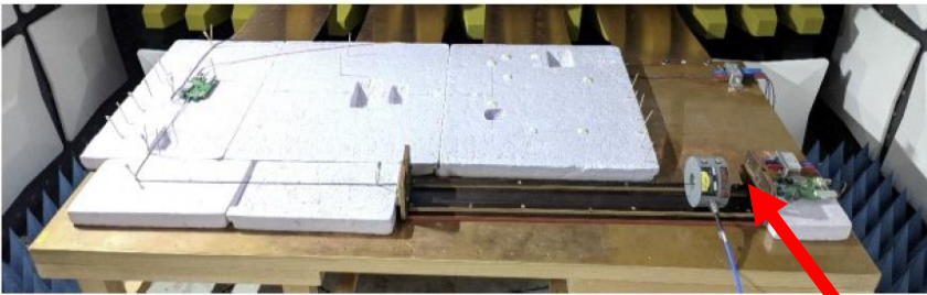
Test set-up, complete arrangement for test channel 2 (2 m), Deserializor is DUT
