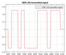
In case there is a high risk that channels may have deep notches (zeroes) in the frequency response near the frequencies of the LS signals, LS signals can be updated to have more widespread spectrum.
