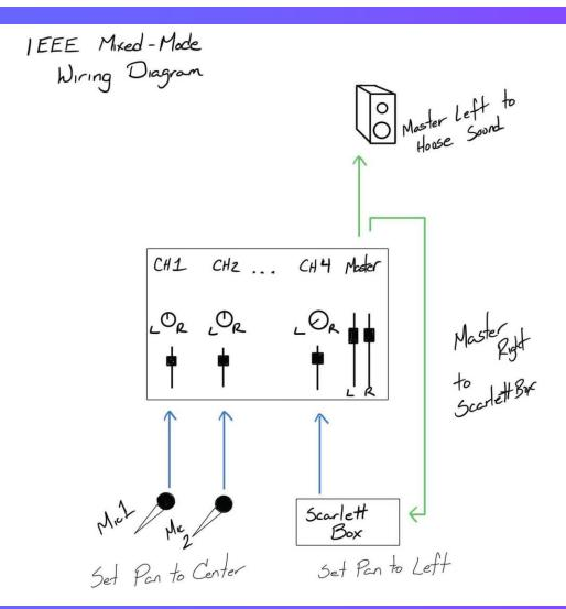
This wiring diagram is provided to assist the AV Engineer at the venue.
