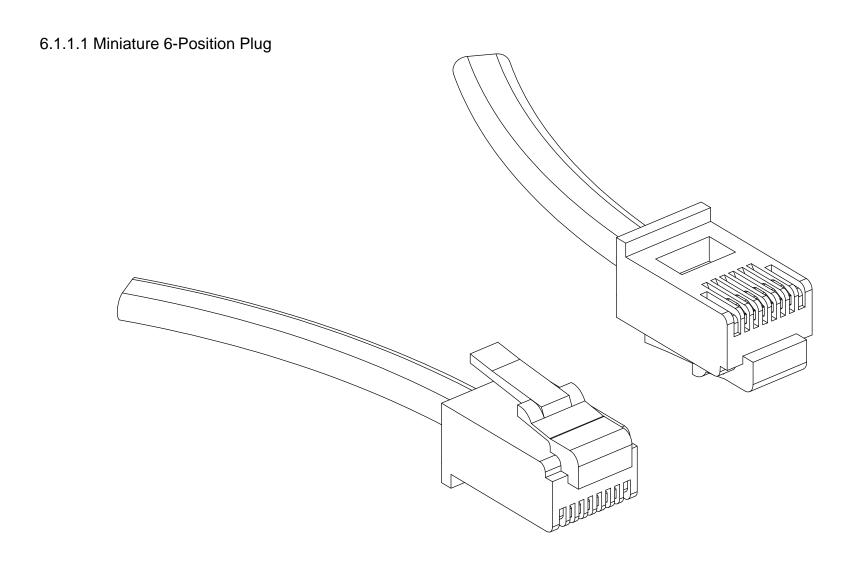
**NOTE:** This plug is depicted equipped with 4 contacts: it may be fabricated with its full 6 contact capability.
