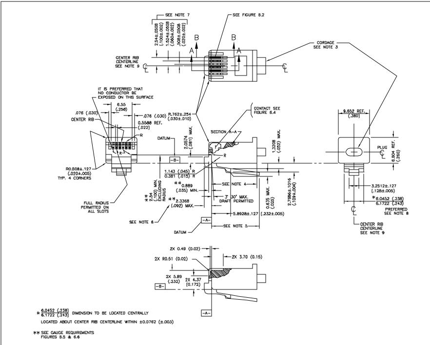
Figure 6.2 6-Position Plug Mechanical Specification
