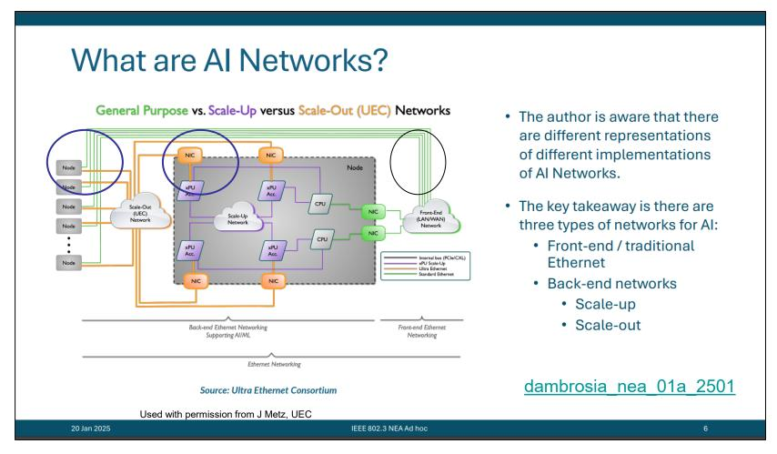
Applications for early adoption of short-reach 200G PHYs include Scale-Out & Scale-Up Networks in Al clusters. Applications can also include the Front-End Network/traditional Ethernet.
