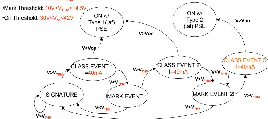
Class Event 3 exists to create a defined behavior for Type 2(.at) PDs when pinged repeatedly. This allows future expansion of the classification mechanism with a known response from Type 2(.at) PDs.
