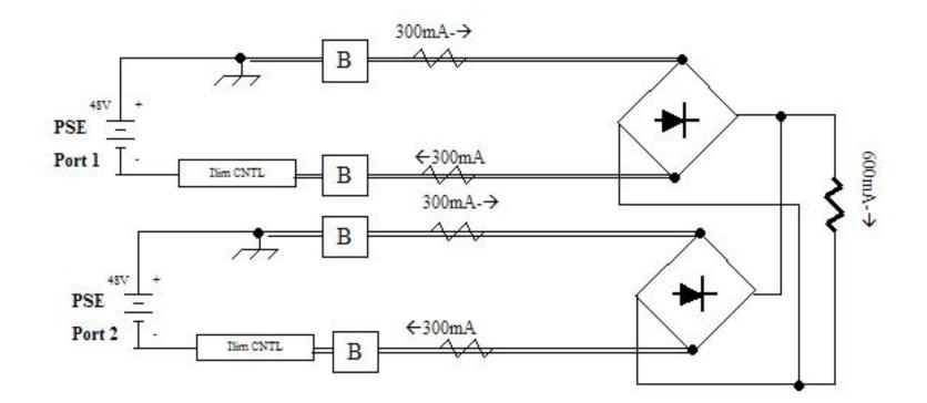
• 4-Pair system requires active balancing on **both the top and bottom** power supply rails.
