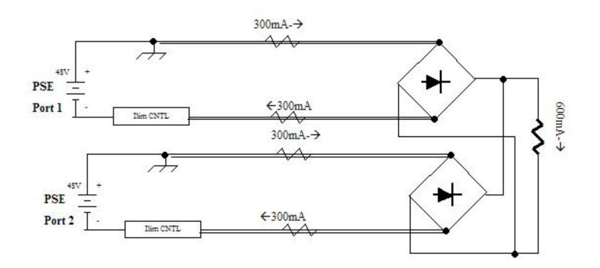
• In this system, current is balanced only because voltage and resistance of system are matched.
