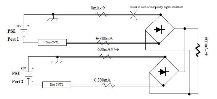
• System resistance mismatch of a just few ohms can offset current enough to throw one port into current limit, therefore shutting down PD.
