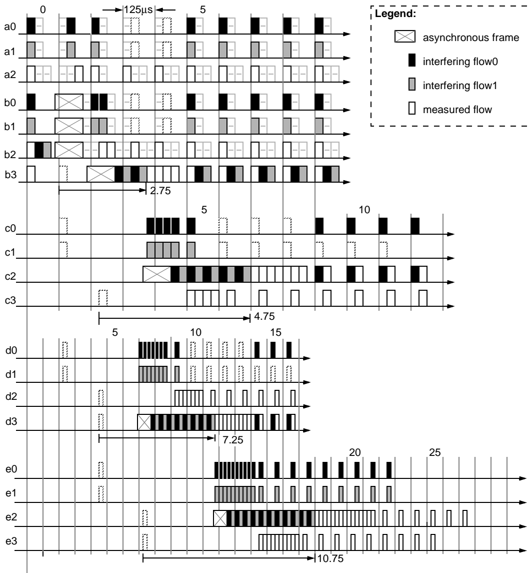
Figure F.12—Three-source bunching; variable-rate output-queue bridges
