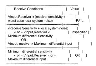
As an unavoidable consequence of the requirements for the setting of the SIGNAL\_DETECT parameter, implementations must provide adequate margin between the input optical power level at which the SIGNAL\_DETECT parameter is set to OK, and the inherent noise level of the PMD due to cross talk,
