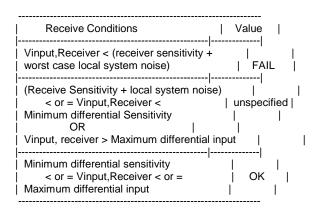
As an unavoidable consequence of the requirements for the setting of the SIGNAL\_DETECT parameter, implementations must provide adequate margin between the input optical power level at which the SIGNAL\_DETECT parameter is set to OK, and the inherent noise level of the PMD due to cross talk,
