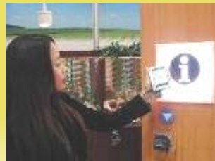
Infra to Mobile, VLCC (Keio Univ., NEC, Toshiba, Sony, Matsushita, Casio etc.) (4.8kbps, illuminations, visible light ID, sign board, applications based on JEITA)
